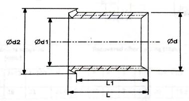
The material used for the End sleeves should be fire retardant/ Self-Extinguishing as per IS:11731 or any other equivalent DIN, IEC.
