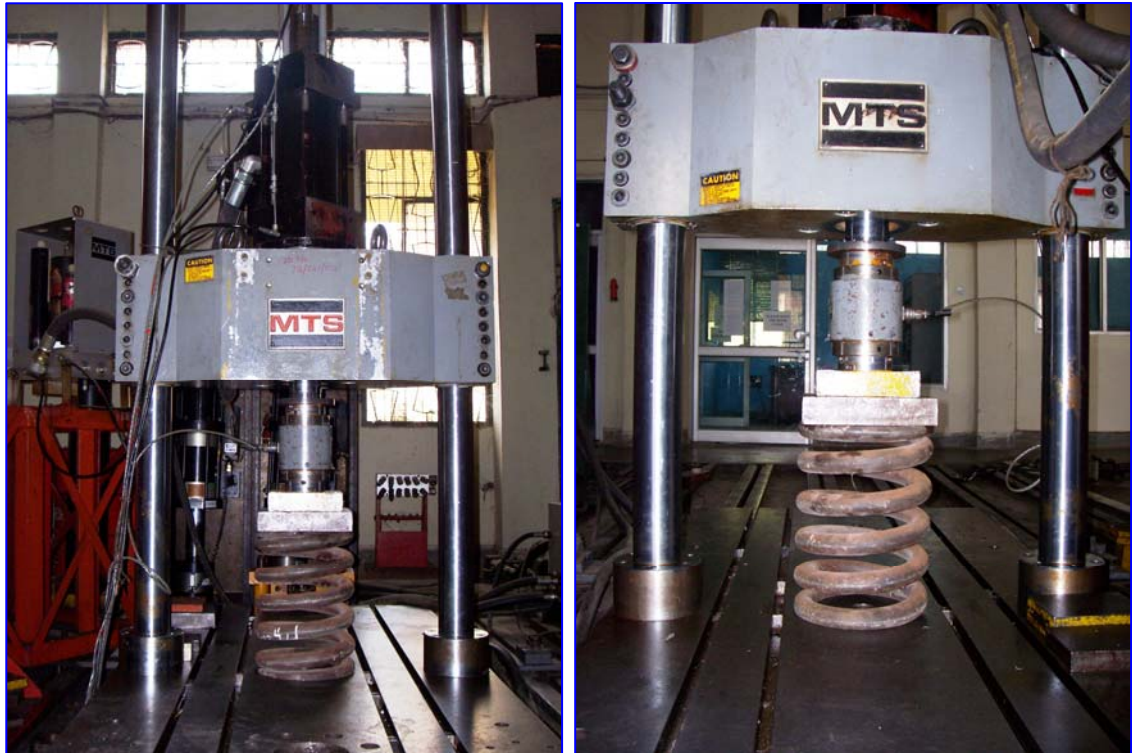
Fatigue Testing Setup for Locomotive Springs
