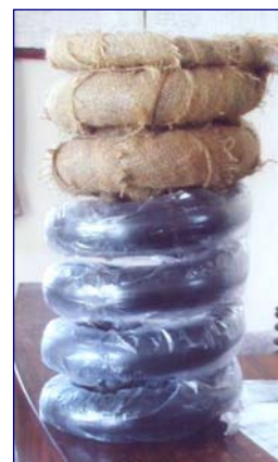
Spring covered with Polythene Sleeve & wrapped with Protective Jute Strip (shown partially covered)
