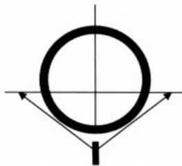
Possible installation position of the Pressure Sensor
