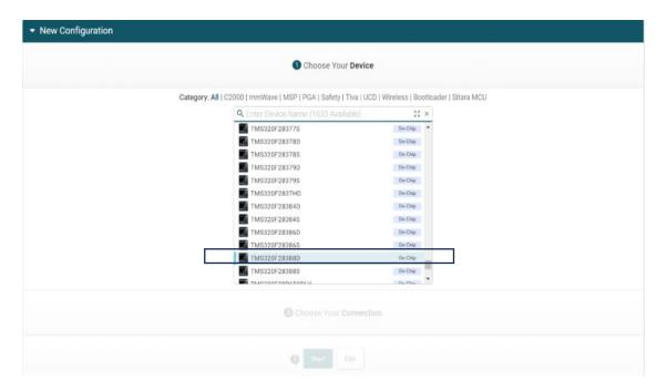
3. After selecting the Device, choose the type of connection between the device and the tool i.e.: Texas instruments XDS100v3 Debug Probe and click on "Start" to choose the file to be programmed.
