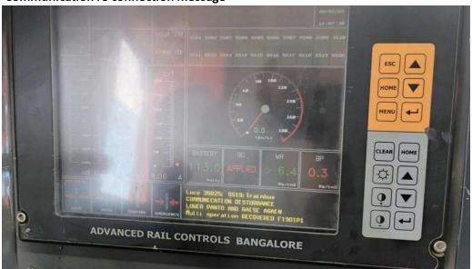
**4.ARC FSK UNIT MOUNTED INSIDE LOCO**
