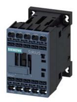
Contactor relay for railway 3 NO + 1 NC DC 72-125V, 0,7...1,25\*US, with integrated varistor Size S00, Spring-type terminal suitable for PLC outputs
